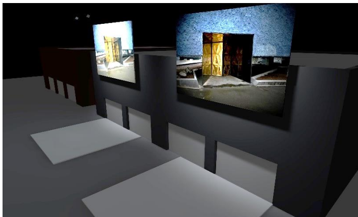
Figure 2: The left advertising panel displays 30% higher luminosity than the right advertising panel. Both panels receive equal illumination. Novljan, T., 3D simulation, Dialux Evo 9.1, 2020.
